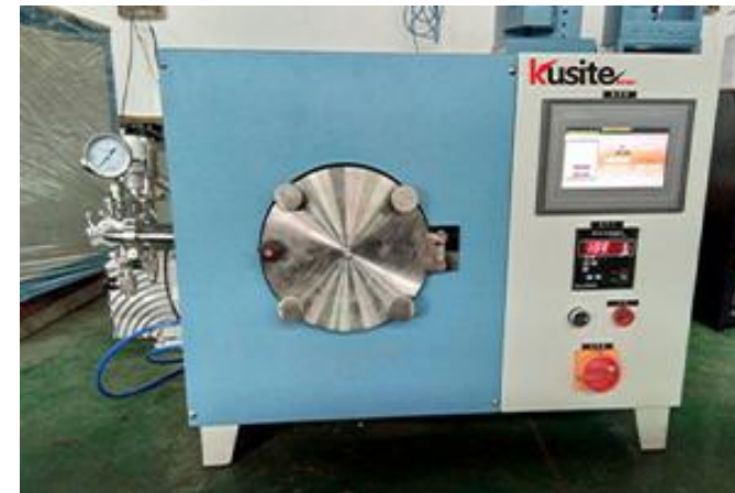
Rapid Annealing Furnace
